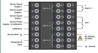
Alarm-2 is only dedicated to the retransmission current output. The indicator outputs pressure as a 4-20mA signal on the Alarm-2 current loop, with 4mA set at the dL value and 20mA set at the dH value. Configure dL and dH in the configuration section.
