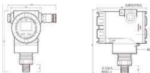
HL 3151T Series of directly mounted intelligent pressure / absolute pressure transmitter appearance size diagram
