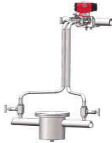
Pipe Differential Pressure Measurement
