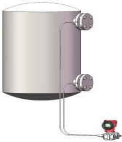
Tank Liquid Level Measurement
